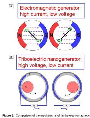
Figure 3. Comparison of the mechanisms of (a) the electromagnetic generator (EMG) based on Faraday's Law of electromagnetic induction and (b) the triboelectric nanogenerator (TENG) that is based on a combination of triboelectrification and electrostatic induction effects. EMG has the characteristic of high current but low voltage, and TENG has a high output voltage but low current. Both EMG and TENG can be applied in tandem.
